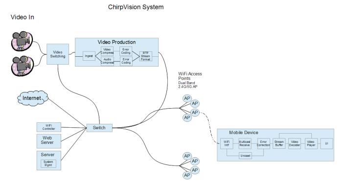
The compressed video and audio streams are created by adding error codes and timestamps. The error codes and timestamps are used as part of the Forward Error Correction (FEC) performed on the mobile device, providing means to detect and correct data errors inflicted during transmission. Streams are formed into standard Ethernet packets that are optimized to match the data format of the compressed stream.
